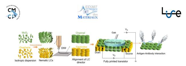
**Project concept**. Electrochemically exfoliated  $MoS_2$  and graphene nanosheets will be stabilized in water and concentrated into LC inks that will be further printed to make a FET biosensor. An Ag/AgCl reference electrode will be used as a gate electrode to apply bias. Anti-Salmonella antibodies will be immobilized on the channel for detecting Salmonella Infantis thanks to the antigen-antibody interaction.
