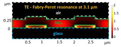
Figure 2 Absorption map for a NC film coupled to a metallic grating
