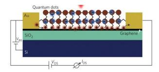
Figure 1 Schematic of a phototransistor where the channel is made of nanocrystal sensitized graphene
